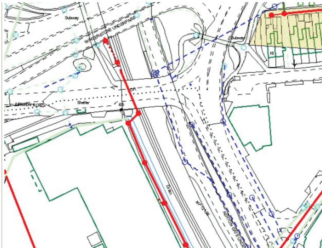
Figure 5: Existing Foul Sewer appears to lie below location of proposed Dn Portbury line
